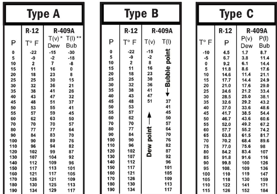
Pressure is on the left, and the columns are temperatures. For blends, there are two columns for dew-point temperature and bubble-point temperature at each pressure.
