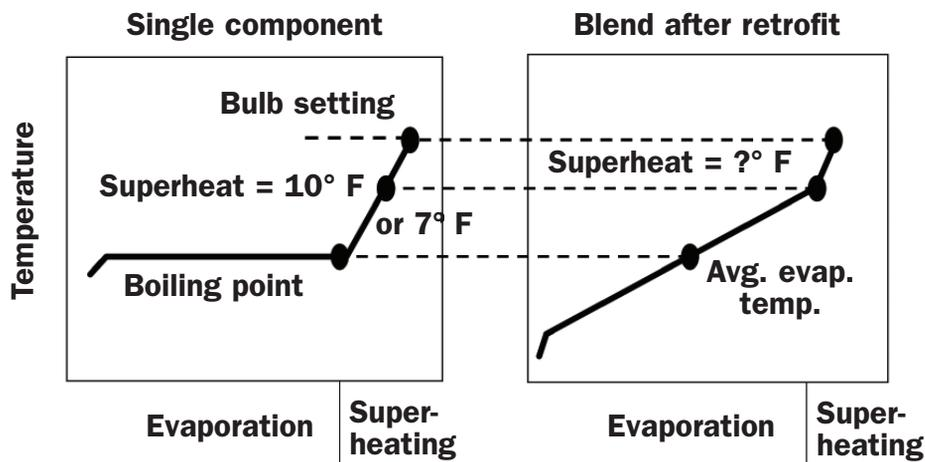
**TXV superheat settings can be affected by temperature glide. This example shows an original superheat setting of 10° F before and after a retrofit to a high-glide blend. The glide allows saturated vapor to move closer to the TXV bulb. This example also considers an original setting of 7° F and a retrofit blend with 14° F of glide, which will eliminate any measurable superheat and allow the valve to flood liquid through.**
