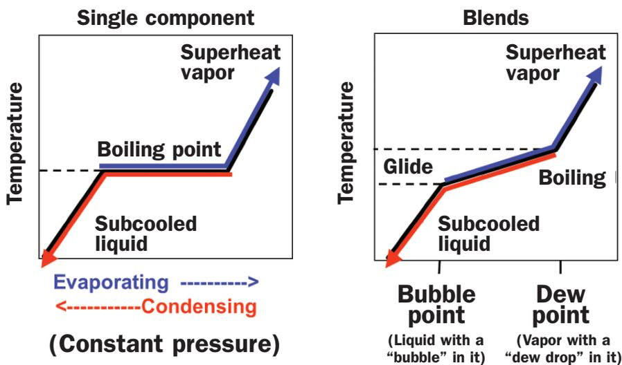
Single-component refrigerants boil at one temperature, and superheat or subcool measurements are compared to that boiling point. Blends change temperature while boiling or condensing, so the end points of the glide must be known in order to calculate superheat or subcool temperature.
